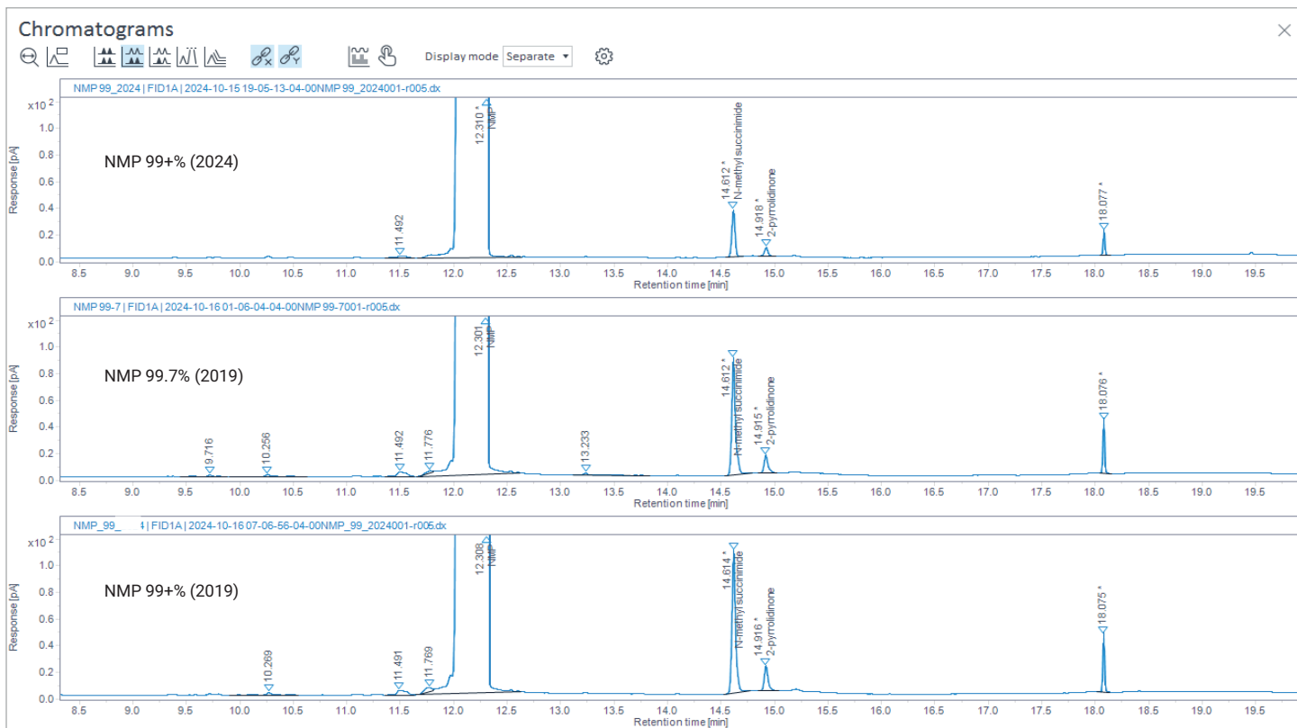
Figure 3. Normalized chromatograms of commercially available solvents, analyzed on an Agilent J&W DB-23 column.
