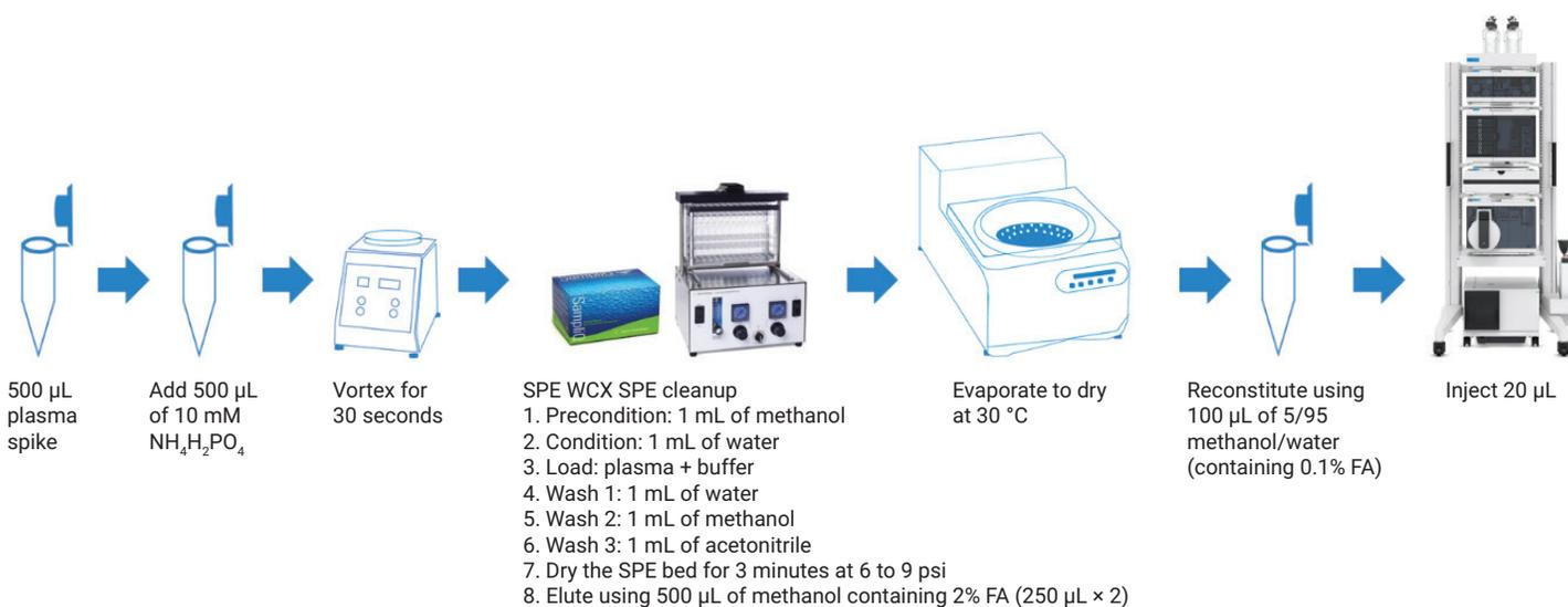
**Figure 1.** Agilent PPM-48 based SPE workflow for sensitive measurement of MN, NMN, and 3-MT in plasma using the Agilent Ultivo LC/TQ.
