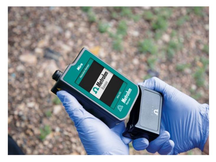
This application is an excellent illustration of two important functions of the MIRA DS handheld Raman system. A good way to characterize Raman sampling is, «If you can see it, Raman can identify it.» Raman also excels at through-container sampling, meaning that information about a material can be collected with no sample contact. This may not be crucial for a sample like Norco®, but during encounters with synthetic opioids, which can be deadly in microdoses, it is essential.
