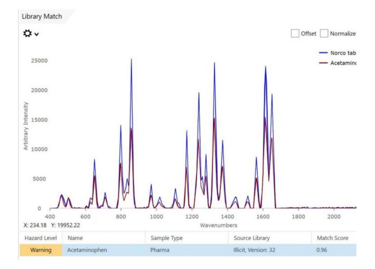
Figure 1. Mira Cal DS spectrum of Norco® tablet with acetaminophen library match supported by high HQI = 0.96.
