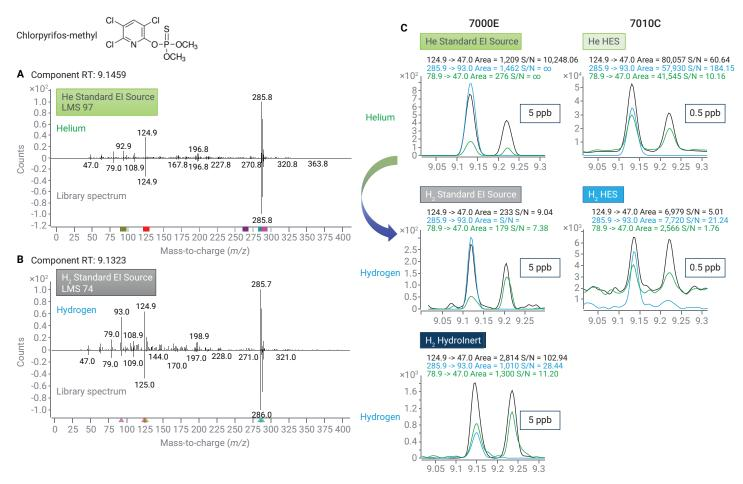
Figure 5. Mass spectra and MRM chromatograms for chlorpyrifos-methyl acquired with helium and hydrogen using the standard El source, the HydroInert, and the HES.
