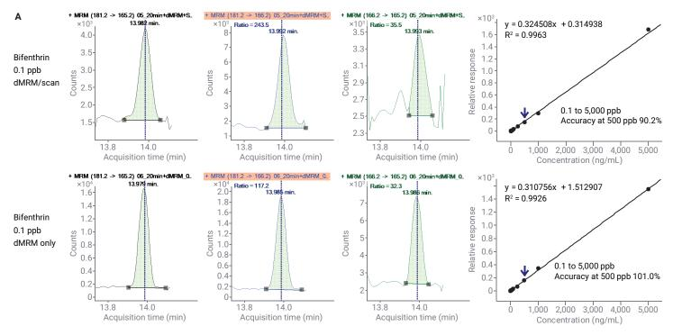
Figure 8A. Quantifier and qualifier ion profiles and matrix-matched calibration curves over 0.1 to 5,000 ppb for bifenthrin spiked at 100 ppb in cayenne pepper with the Agilent 7000E GC/TQ in simultaneous dMRM/scan and dMRM only data acquisition modes.
