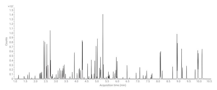
Figure 1. TIC of the 50  $\mu$ g/mL calibration standard showing separation in under 10 minutes
