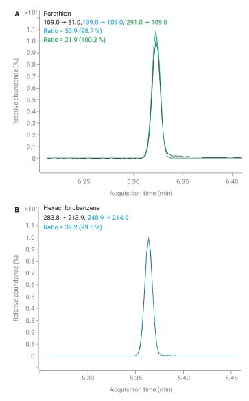
**Figure 3.** Overlays of MRM transition EICs for (A) parathion and (B) hexachlorobenzene, when using  $H_2$  carrier gas and the Agilent HydroInert source on a GC/MS/MS system, showing retention of key functional groups in the presence of  $H_2$ .
