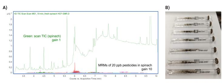
Figure 8. (A) TIC of a full scan chromatogram acquired for spinach extract and the MRM TIC for 20 ppb pesticides. (B) The GC inlet liners replaced after 100 injections when analyzing spinach extract during the robustness evaluation.
