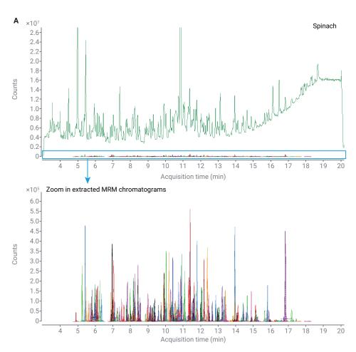
Figure 5A. Scan (on top) and dMRM (magnified on the bottom) TIC acquired in simultaneous dMRM/scan data acquisition mode for spinach extract.
