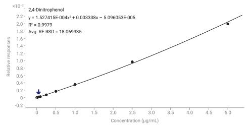
Figure 6. Alternate calibration curve for 2,4-dinitrophenol with a quadradic curve fit 0.05 to 5  $\mu$ g/mL. R<sup>2</sup> = 0.9979. Calibration points 1, 2, 3, and 11 are excluded.
