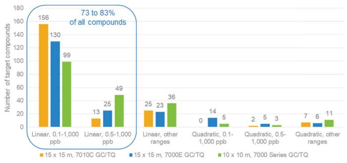
**Figure 6.** Calibration performance for the 203 pesticides with the 10-minute methods using the conventional 15 × 15 m configuration, coupled with the Agilent 7010C and 7000E triple quadrupole GC/MS systems, and the minibore 10 × 10 m configuration, coupled with the Agilent 7000 series triple quadrupole GC/MS in spinach. The graph shows the number of compounds and their calibration ranges.
