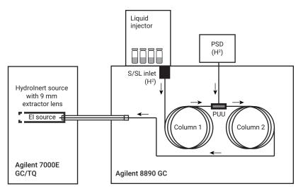
Figure 1. System configuration.
