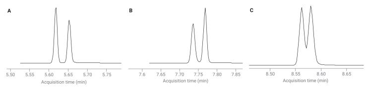
**Figure 2.** Midlevel standard (5  $\mu$ g/mL) MRM transition extracted ion chromatograms (EICs) for critical isomer pairs: (A) phenanthrene and anthracene (MRM transition of 178.1  $\rightarrow$  152.1 *m/z*); (B) benz[a]anthracene and chrysene (228.1  $\rightarrow$  226.1 *m/z*); (C) benzo(b)fluoranthene and benzo(k)fluoranthene (252.1  $\rightarrow$  250.1 *m/z*).
