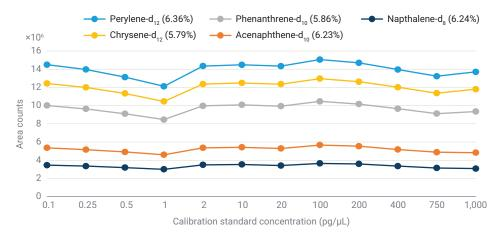
Figure 3. ISTD response over the calibration range.
