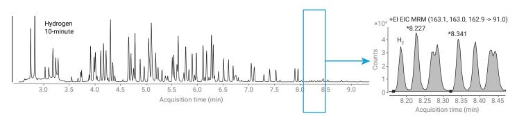
Figure 4. MRM chromatograms for a mixture of 103 pesticides acquired with hydrogen with the 10-minute method using a 10 m × 10 m minibore configuration.
