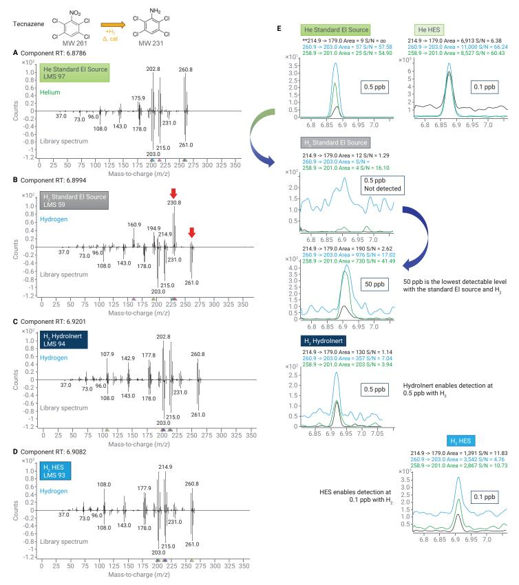
Figure 6. Mass spectra and MRM chromatograms for tecnazene acquired with helium and hydrogen using the standard El source, the HydroInert, and the HES.
