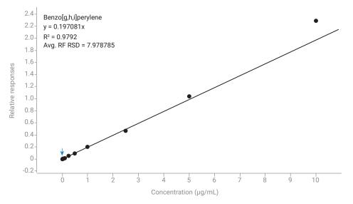
Figure 7. Avg RF calibration curve for benzo[g,h,i]perylene 0.005 to 10 µg/mL. Avg RF RSD = 7.98.
