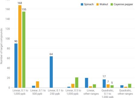
**Figure 11.** Calibration performance for the 203 pesticides with the 7000E and 7010C GC/TQ in spinach. The graph shows the number of compounds and their calibration ranges.
