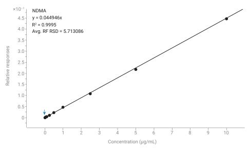
Figure 9. Calibration curve for NDMA. 0.01 to 10 µg/mL. Avg. RF RSD = 5.71. Calibration point 1 excluded.
