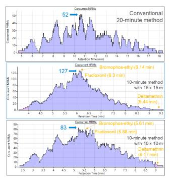
**Figure 2.** The distribution of 614 dMRM transitions with the 20-minute conventional pesticide analysis, the 10-minute analysis employing the conventional  $15 \times 15$  m configuration, and the 10-minute method employing the minibore  $10 \times 10$  m column configuration.
