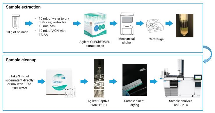
Figure 2. Sample preparation flowchart including traditional Agilent QuEChERS extraction, followed by Agilent Captiva EMR pass-through cleanup.
