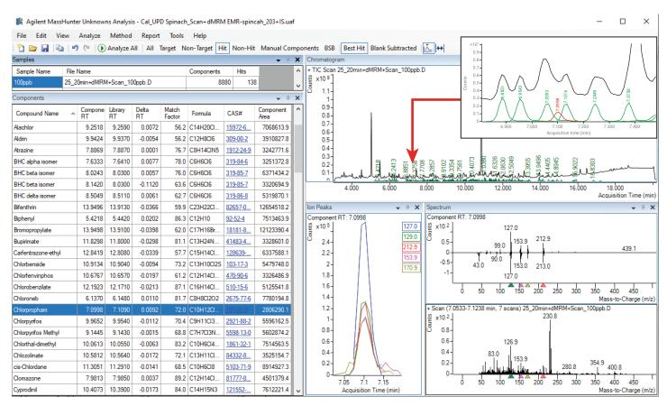
**Figure 6.** A partial list of search results for spinach extract spiked with a pesticide mixture at 100 ppb against a retention time-locked spectral library. Chlorpropham is selected in the components table and its extracted ion chromatograms and corresponding spectral information are shown on the lower right. The data were acquired with the 7000E GC/TQ in simultaneous dMRM/scan mode.
