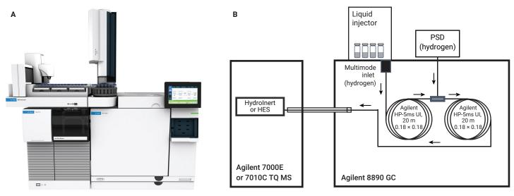
Figure 1. The Agilent 8890/7000E and 8890/7010C GC/TQ system (A) and system configuration (B).
