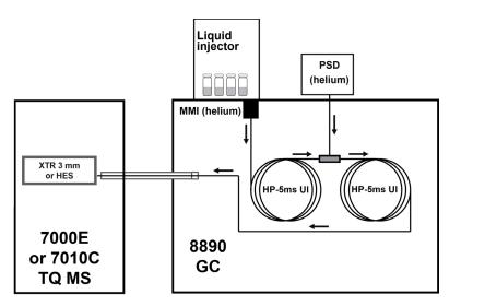
Figure 1. The Agilent GC/TQ system featuring two utilized midcolumn backflush configurations (right).
