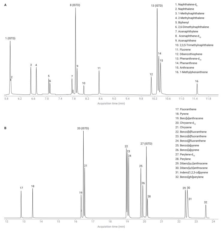
Figure 2. MRM TIC of 27 PAHs at 100 pg/µL and five ISTDs at 500 pg/µL.
