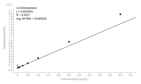
Figure 5. Avg RF calibration curve for challenging analyte 2,4-dinitrophenol 0.05 to 5  $\mu$ g/mL. Avg. RF RSD = 18.07. Calibration points 1, 2, 3, and 11 are excluded.
