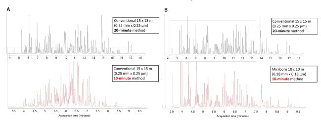
Figure 4. MRM total ion current chromatograms (TIC) or a mixture of 203 pesticides acquired with (A) the conventional  $15 \times 15$  m configuration and (B) with the minibore  $10 \times 10$  m configuration.
