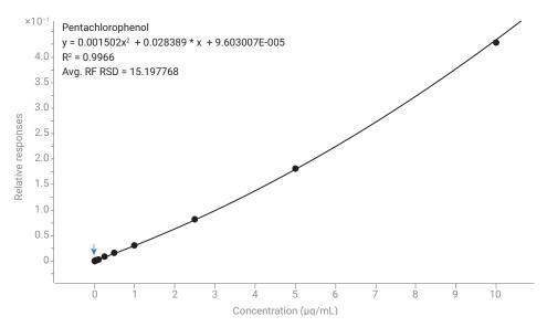
Figure 8. Calibration curve for pentachlorophenol 0.01 to 10  $\mu$ g/mL. R<sup>2</sup> = 0.9966. Calibration point 1 excluded.
