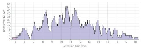
Figure 2. The distribution of 614 MRM transitions with up to 52 concurrent MRMs monitored during the analysis enabling most efficient dwell time distribution.
