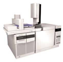
Agilent is leading the way by introducing IDL, Instrument Detection Limit, as a new metric for meaningful indication of system sensitivity. In MS/MS baselines with very little noise, the dubious selection of noise region highly influences and inflates the S/N values. IDL is a true reflection of the whole system performance and a more accurate expression of achievable detection limit than the customary S/N specification.
