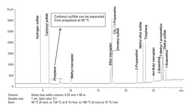
Figure 3. A complete separation of COS from propylene without matrix interference.
