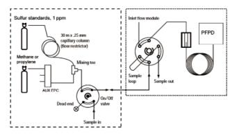
Figure 1. The configuration of the gas blending and GC-PFPD system.
