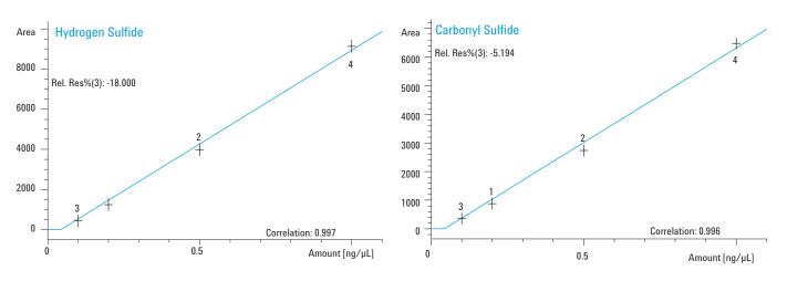
Figure 5. Calibration curves for hydrogen sulfide and carbonyl sulfide.
