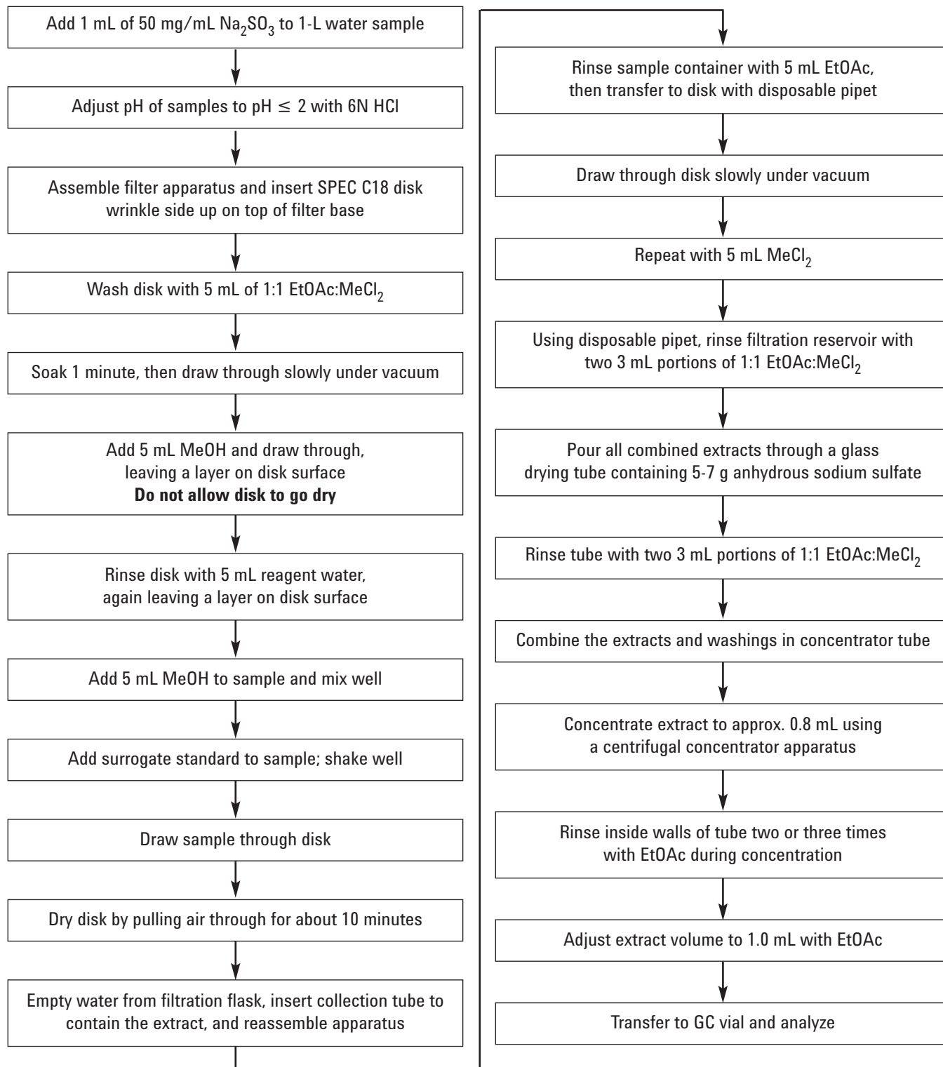
Figure 1. Flow chart for the extraction of chlorinated pesticides in water.
