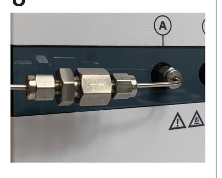
No checkout sample is included with the Micro GC. Connect an appropriate sample gas or calibration gas.
