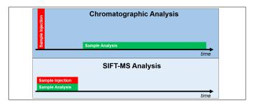
**Figure 2.** Graphical representation of the different sampleinjection and analysis requirements of chromatographic techniques and SIFT-MS.
