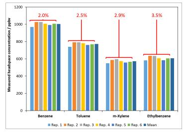
**Figure 5.** SIFT-MS measurement repeatability (six replicates) for direct water headspace analysis of 250-ppb solutions of benzene, toluene, ethylbenzene, and m-xylene. The mean concentration is also shown.
