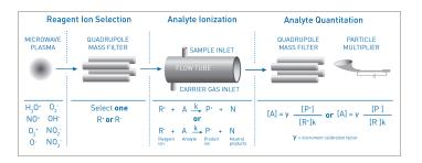
**Figure 1.** Schematic diagram of SIFT-MS – a direct chemicalionization analytical technique. At least 12 samples per hour are analyzed using this approach without compromising the ability to selectively analyze isomeric ethylbenzene and total xylenes.
