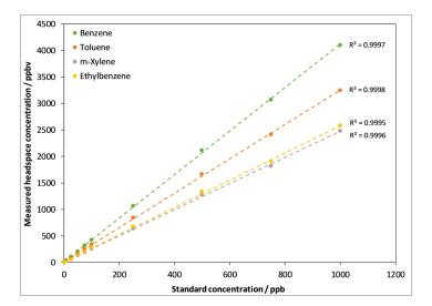
**Figure 4.** SIFT-MS measurement linearity for direct water headspace analysis of benzene, toluene, ethylbenzene, and m-xylene
