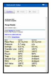
Instrument Status Screen -Provides real-time monitoring of the analytical process including active method, current mode and a complete list of current and set instrument parameters.
