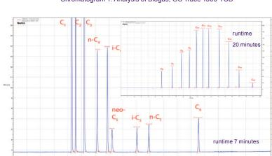
Chromatogram 2. Extended Biogas analysis, GC Trace 1300-FID
