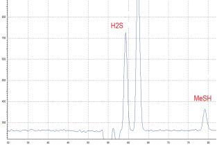
Chromatogram 5: 0.8 ppm  $\rm H_2S,$  1.3 ppm COS and 350 ppb MeSH in Biogas
