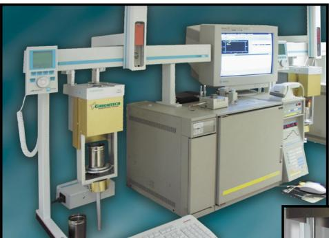
Fig. 3. Installation of a parallel BAKER system on 2 gas chromatographs
