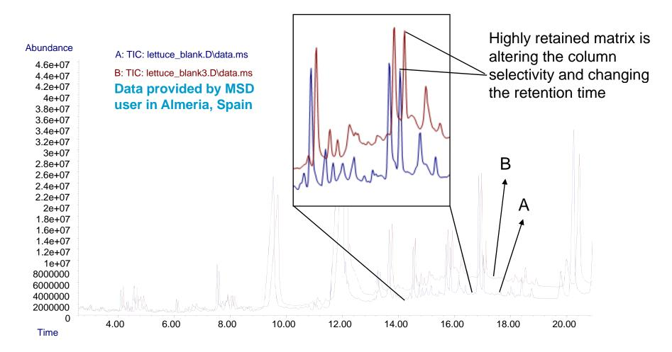
Overlay of two chromatograms of a blank extract injected BEFORE (A) and AFTER (B) three injections without backflush
