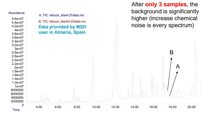
Overlay of two chromatograms of a blank extract injected BEFORE (A) and AFTER (B) three injections without backflush
