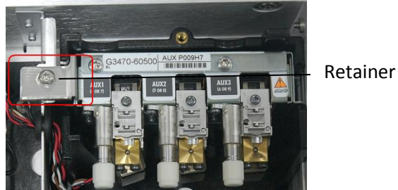
Figure 9 Installing the Aux EPC
