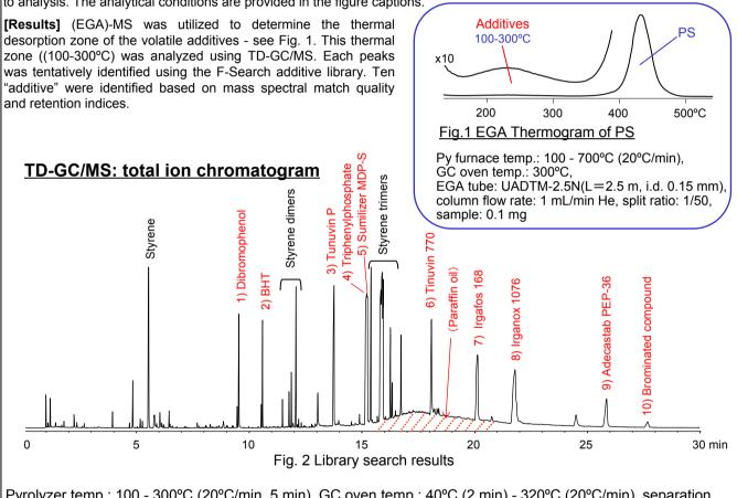
Pyrolyzer temp.: 100 - 300°C (20°C/min, 5 min), GC oven temp.: 40°C (2 min) - 320°C (20°C/min), separation column: Ultra ALLOY<sup>+</sup>-5 (5% diphenyl 95% dimethylpolysiloxane) (L=30 m, i.d.=0.25 mm, df=0.05 μm), column flow rate: 1 mL/min He, split ratio: 1/20, scan rate: 2 scans/sec, scan range: 29 - 810 (m/z), sample: 1 mg
