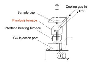
Fig. 1. Structure of Double-Shot Pyrolyzer
