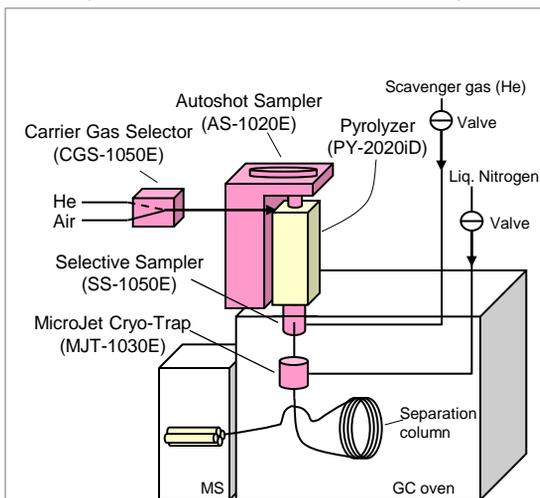
Figure 1. Automated oxidative pyrolysis and pyrogram acquisition system
