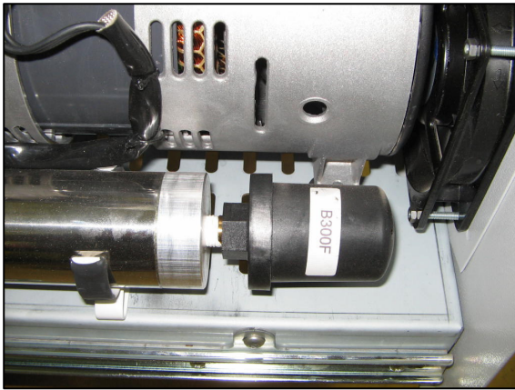
Compressor 2750 Intake filter
