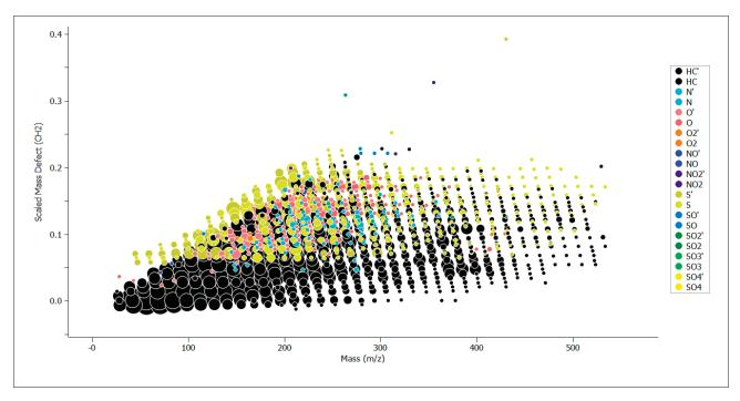
Kendrick's scaled Mass Defect Plot of Crude Oil Sample with heteroatomic species classified by color (see legend, note ' indicates odd electron ion).
