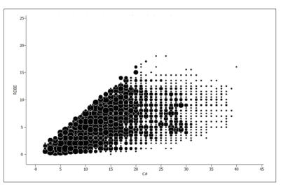
**RDBE** versus Carbon Number Plot of Crude Oil Sample shows the distribution of heavy versus light compounds by class (HC in this case).
