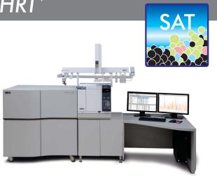
Particularly useful in Petroleomics and Environmental workflows, SAT provides extensive functionality built on top of standard mass defect plots, as well as new van Krevelen and Degree of Unsaturation (RDBE versus C#) plots.
