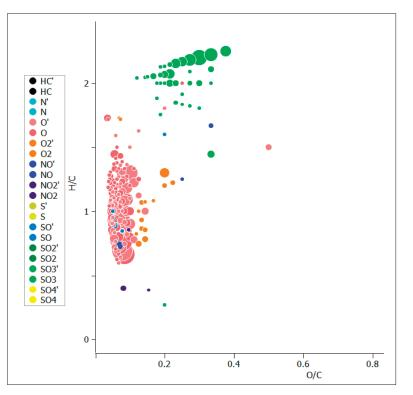
Van Krevelen Plot of Crude Oil Sample shows the shows the ratio of H/C versus O/C for N and O containing species.
