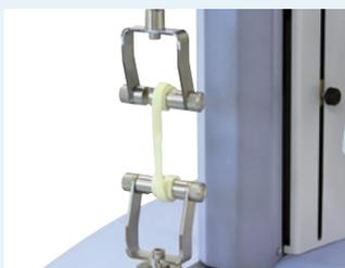
Tensile and Shearing Test for Noodles
