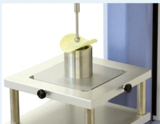
Potato Chip Breakage Test
