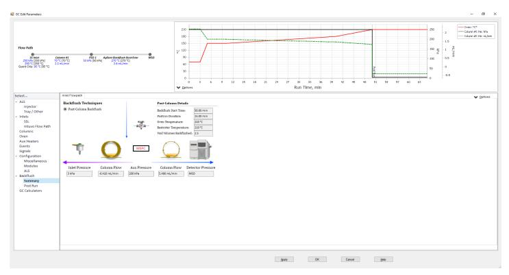
Figure 1. Screenshot of backflush calculator in Agilent MassHunter Acquisition software.
