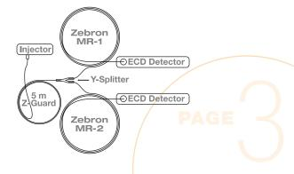
By making one injection and splitting the sample into two columns, both Procedure A and Procedure B can be accomplished at the same time. If a calibration curve is run before each batch of samples and a suitable calibration check is run after each batch of samples to verify the stability of the calibration, then Procedure C could also be run at the same time. The main obstacle of using this type of system is to use one oven program to separate the target analytes on two column phases.
