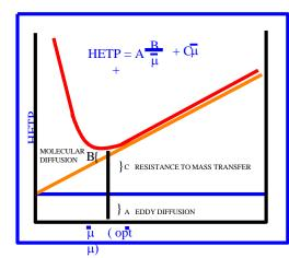
Efficiency is a function of the carrier gas linear velocity or flow rate.
