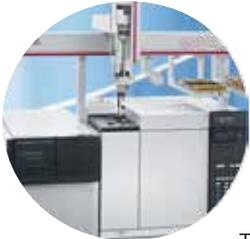
The GERSTEL MultiPurpose Sampler (MPS robotic) Dual Head version, automates all steps including liquid handling, liquid-liquid extraction, evaporative concentration of extracts, change to a GC compatible solvent and derivatization of the analytes. If the MPS is integrated with a GC/MS system, the entire process including GC/MS analysis is automated and automatically optimized for highest productivity and throughput.
