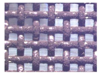
Figure 2. Light Microscope photograph of CMS bonded to a mesh screen (40X)
