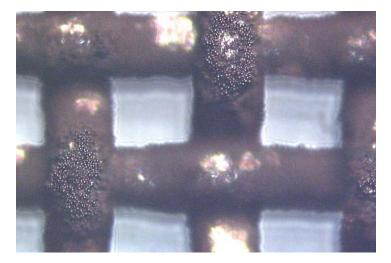
Figure 3. Light Microscope photograph of CMS bonded to a mesh screen (100X)
