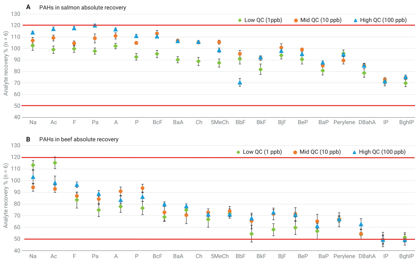
Figure 6-8. PAH recovery in (A) salmon and (B) beef using the optimized sample preparation procedure.
