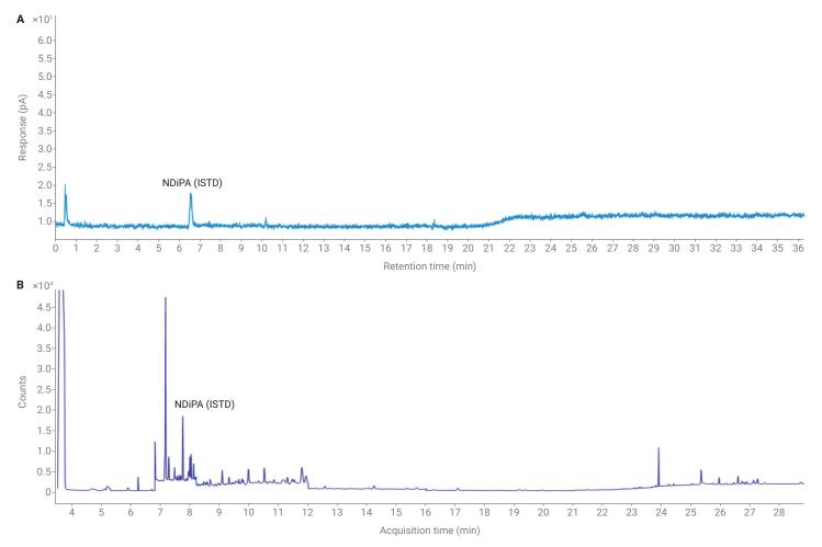
Figure 6. (A) Chromatogram of the real sample based on NCD. (B) Chromatogram of the same real sample based on Agilent 5977B MSD SIM mode on an Agilent DB-WAX 30 m  $\times$  0.25 mm, 0.25  $\mu$ m column. The GC parameters of inlet and injection size are the same as the NCD method, which is shown in Table 1.
