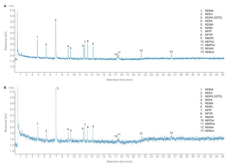
Figure 5. (A) GC chromatogram of a calibration solution at a concentration of 25 µg/L. (B) GC chromatogram of a calibration solution at a concentration of 10 µg/L.
