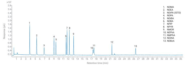
Figure 4. GC/NCD chromatogram of a calibration solution at a concentration of 200 µg/L.
