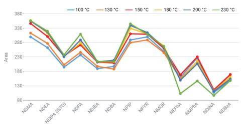
Figure 1. Inlet initial temperature versus peak area for nitrosamine compounds.
