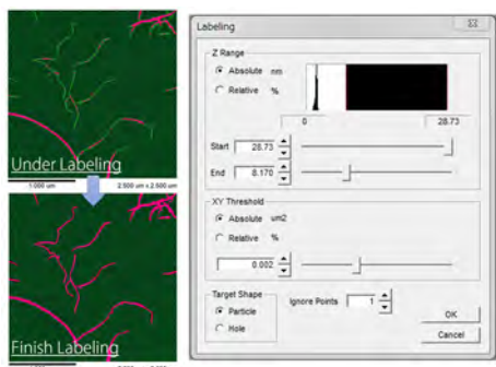
Fig. 6 Particle Extraction Process of Particle Analysis Software
