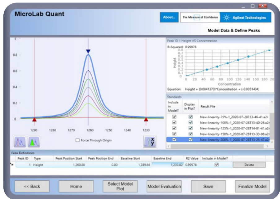
Figure 9. Linearity evaluation of the DialPath sampling module using MicroLab Quant. Calibration curves and correlation coefficient calculations are performed automatically in the software.
