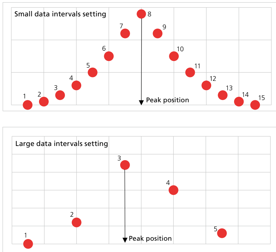
Fig. 3 Illustration of Measurements Obtained by Changing the Data Intervals Setting (Each Dot Indicates One Light Measurement Value)
