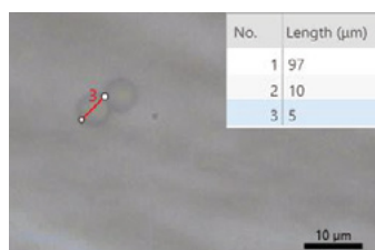
Fig. 5 The measurement of particle size using the length measuring function
