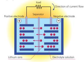
Lithium ions between the layers in the carbon negative electrode material pass through the separator and into the lithium compound (positive electrode material), resulting in a discharging current flow.
