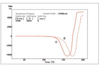
TMA Measurement of Separator Contraction Behavior
