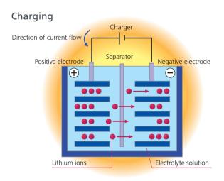
Lithium ions in the lithium compound (positive electrode material) pass through the separator and into the layers in the carbon negative electrode material, resulting in a charging current flow.
