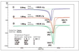
DSC Measurement of Separator Melting
