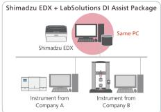
Note 1) Only one Shimadzu instrument can be connected to the PC for controlling Shimadzu instruments.
