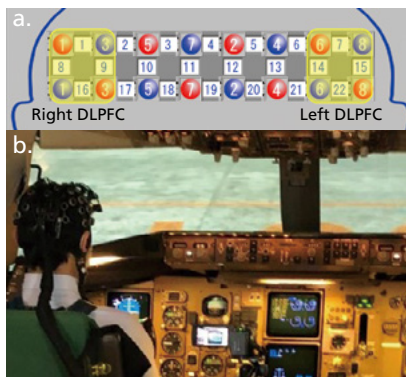
Fig. 1 a. Regions of Interest: Left/Right DLPFC b. Testing Conditions Using the ANA Blue Base Boeing 767-300 Twin Engine Simulator
