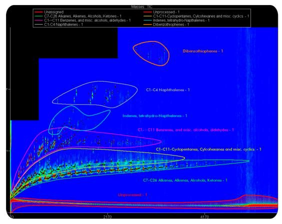
A highly structured GCxGC-TOFMS Contour Plot showing analysis of a Light Crude Oil Standard. This analysis uses variable modulation and classifications to facilitate the characterization of classes of compounds in this complex petroleum based sample.
