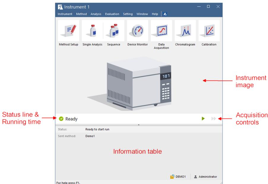
Fig 3: Instrument window
