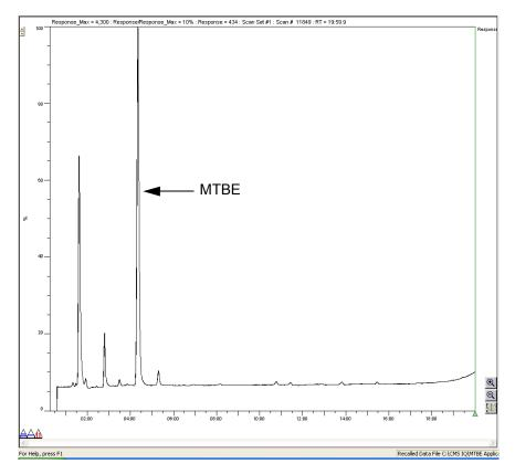
Figure 1 Chromatogram of MTBE at a Concentration of 5.0 ppb
