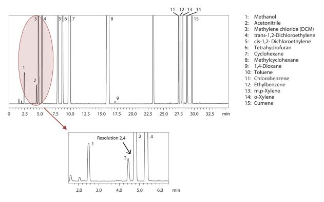
Fig. 3 Chromatogram of WATER-SOLUBLE ARTICLES Class 2A Standard Solution by Procedure A
