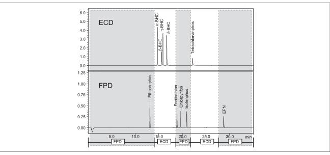
Fig. 2 Chromatograms of Pesticides Obtained by ECD - FPD Switching
