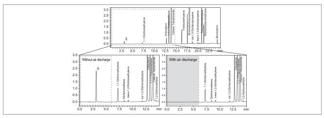
Fig. 4 Chromatograms With and Without Air-Elimination
