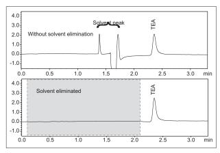
Fig. 3 Chromatograms of With and Without Solvent Elimination
