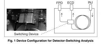
is required for detection of all the pesticide constituents. Here we introduce an e xample of sim ultaneous analysis of a standard solution of pesticides using switching between an FPD (flame photometr ic detector) and ECD (electron capture detector).
