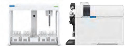
The standard 7800 ICP-MS configuration was used, which consisted of a Micromist glass concentric nebulizer, quartz spray chamber, quartz torch with 2.5 mm id injector, nickel plated copper sampling cone and a nickel skimmer cone. The system is also offered as an ICP-MS Cannabis Analyzer.
