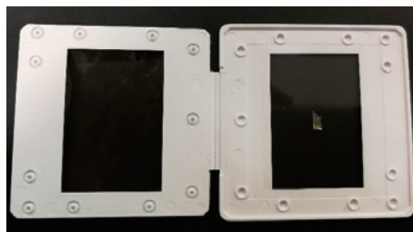
Fig. 4-1 Attach Contaminants to EDXIR-Holder
