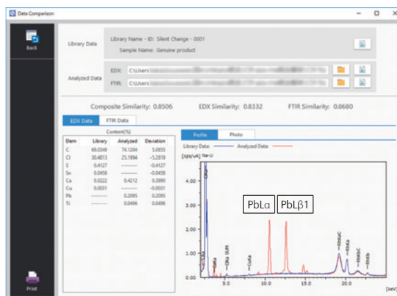
Fig. 9 Data Comparison Results and X-Ray Fluorescence Profiles
