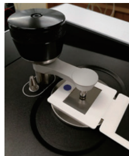
Fig. 4-2 Performing the FTIR Measurement
