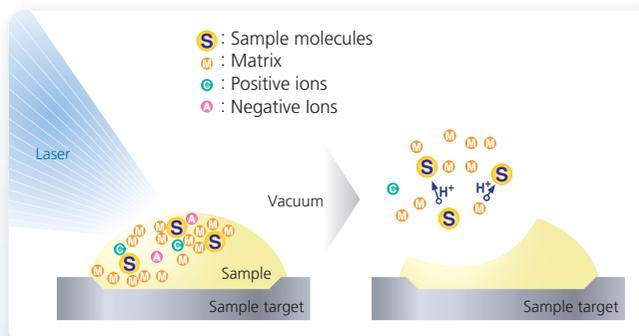
Sample ions are separated and detected based on differences in their mass-to-charge ratio ( $m/z$  value).
