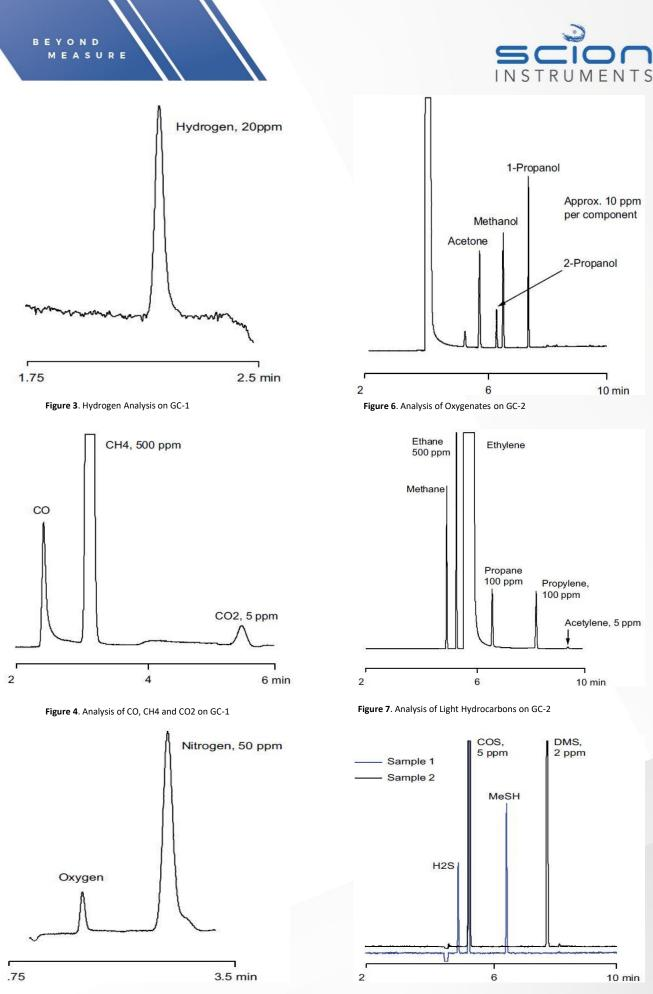
Figure 5. Analysis of O2 and N2 on GC-1
