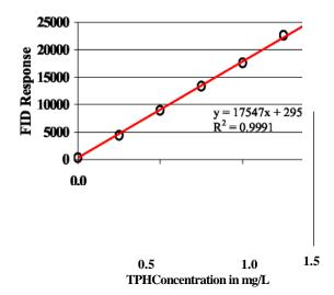
**Figure 3: Low-level TPH calibration plot** – standards with actual TPH-concentrations of 0, 10, 20, 30, 40 & 50 μg/mL were used to obtain this plot
