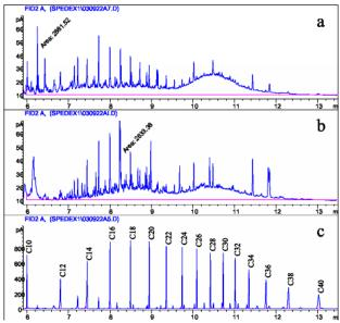
Figure 1: LVI-GC-FID chromatograms – (a) 5  $\mu$ g/mL Standard; (b) 125  $\mu$ g/L TPH extract; and (c) 1  $\mu$ g/mL n-Alkane Florida Mix. The top pair of chromatograms has the same amount of TPH present in the 50- $\mu$ L injection volumes analysed.
