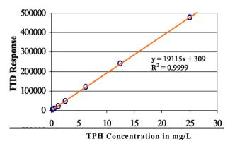
Figure 2: Linear calibration upto 25 mg/L – the TPH-concentration of the standards used were 0, 10, 20, 50, 100, 250, 500 & 1000  $\mu$ g/mL, respectively.
