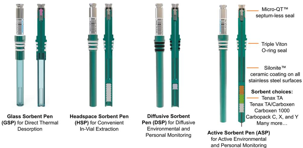
**Sorbent Pen (SP)** schematic, showing the Micro-QT vacuum seal and the internal sorbent bed. The SPs come in four different configurations and can be packed with a variety of sorbents, including multi-component beds of varying physical properties.
