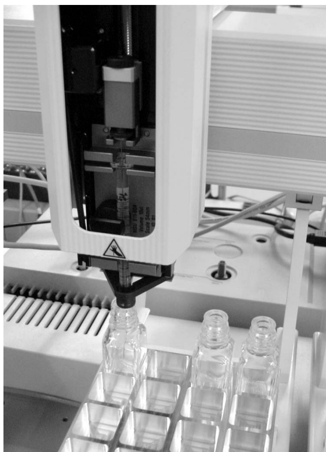
Figure 6. Example of a custom tray developed for custom vials.
