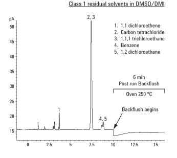
Figure 3. Backflush of Class 1 residual solvents in DMSO/DMI.
