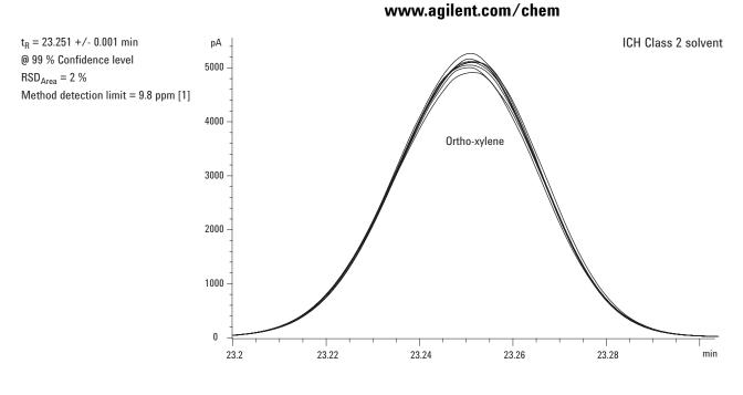
Figure 4. O-xylene (195 ppm), overlay N = 8 (BPR of HS loop @ 5 psi, HS vial pressurized to 20 psi).
