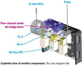
**Exploded view of module components.** You can program the module to automatically change the carrier gas to nitrogen when your GC is not in operation.
