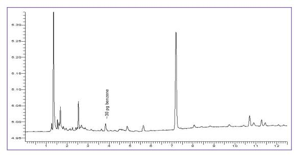
Figure 1: 30 pg of benzene from a sorbent tube. Equivalent to 10 ppt in 1 L of air
