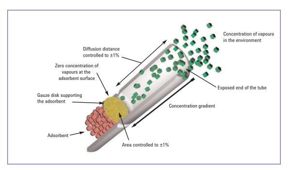
Figure 2: Illustration of diffusive sampling on axial sorbent tubes
