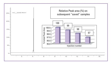
Figure 4: Re-collection and repeat analysis of desorbed toluene
