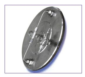
Figure 5: FLEC - Field and Laboratory Emission Cell for materials emission testing
