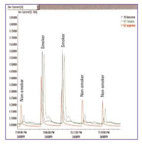
Figure 9: The breath of 5 individuals, 2 smokers and 3 non-smokers, monitoring for benzene, toluene and isoprene
