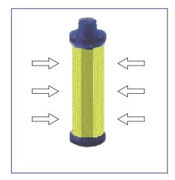
Figure 3: Radial diffusive samplers
