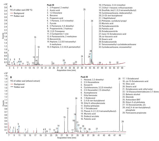
Figure 2. Extractables analysis of a rubber seal using headspace equilibrium temperature of 250 °C (A) and ethanol extraction by MMI GC/MS (B).
