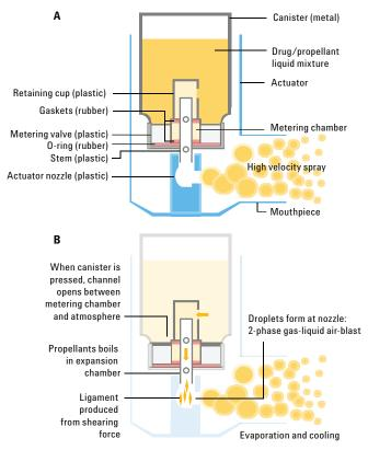
Figure 1. Design of a pressurized metered dosed inhaler (A) and operation of the metering valve (B).
