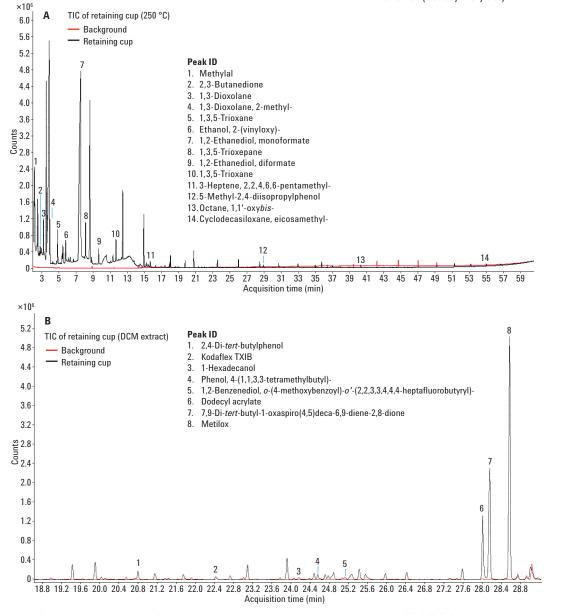
Figure 3. Extractables analysis of a retaining cup using headspace equilibrium temperature of 250 °C (A) and DCM extraction by MMI GC/MS (B).
